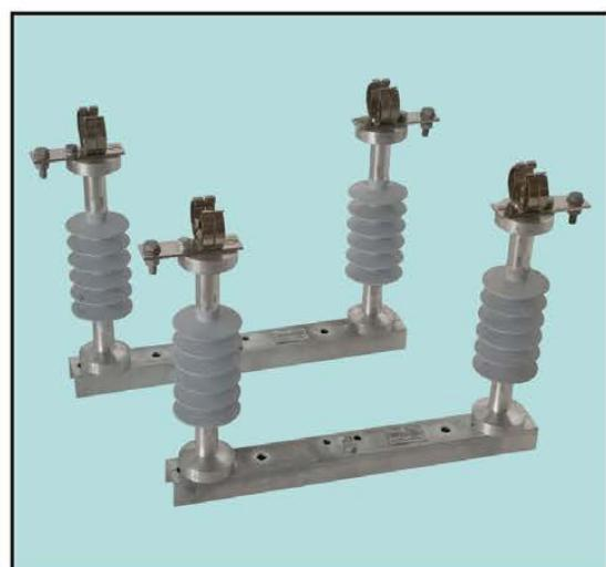
The outdoor high-voltage fuse bases are factory manufactured and tested in accordance with the applicable MKS and IEC standards. They serve as the support for mounting high voltage fuses in pole-mounted transformer substations and overhead transmission lines, which require fuses for overcurrent protection. Silicon insulators are used for insulation. They can be single-pole or three-pole.
